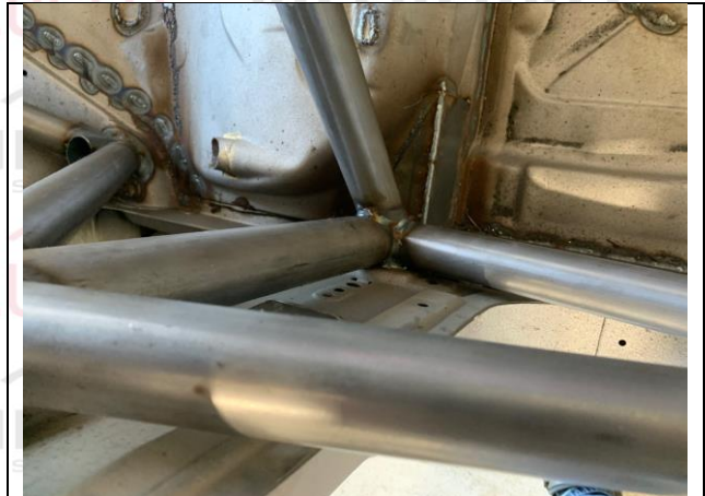
PHOTO 4 MAIN ROLLBAR TO FLOOR ATTACHMENT
