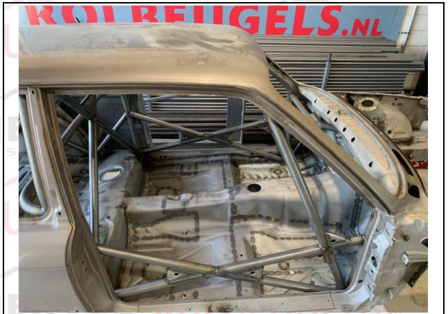
PHOTO 11 ANTI-INTRUSION DOORBAR - CO-DRIVER
