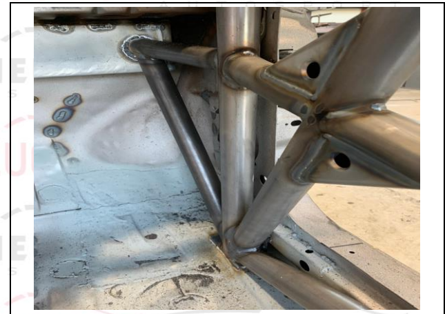
PHOTO 6 FRONT ROLLBAR TO FLOOR ATTACHMENT
