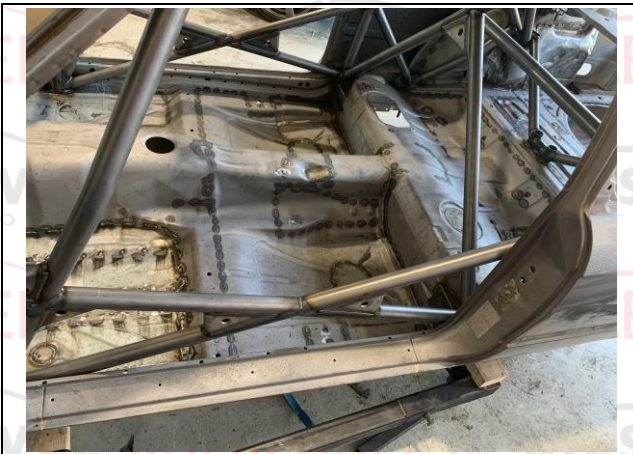
PHOTO 10 ANTI-INTRUSION DOORBAR - DRIVER
