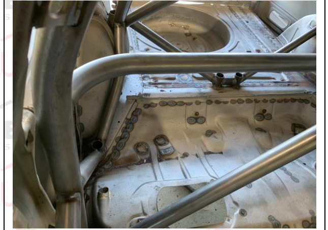
PHOTO 13 SHOULDER HARNESS ATTACHMENT - CO DRIVER
