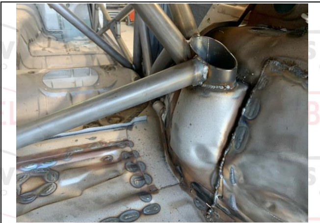
PHOTO 5 REAR BACKSTAY TO BODYSHELL ATTACHMENT
