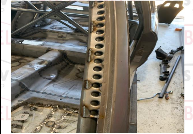
PHOTO 7 FRONT ROLLBAR TO "A" PILLAR ATTACHMENT
