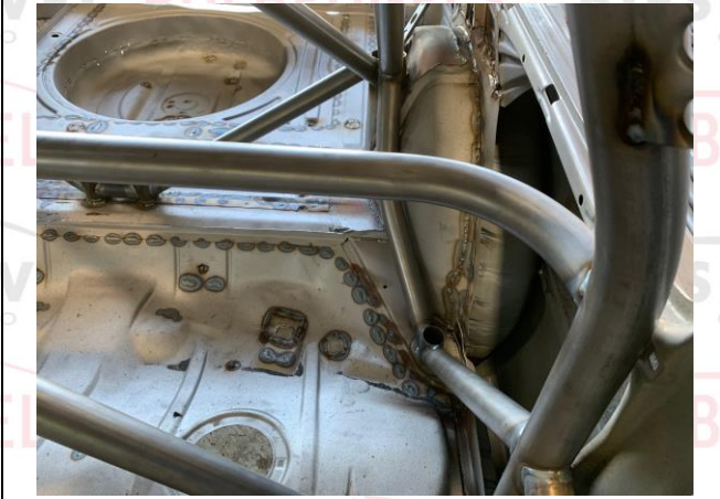
PHOTO 12 SHOULDER HARNESS ATTACHMENT - DRIVER
